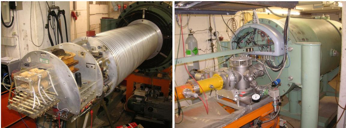
**Figure A.6:** 2 MV Van-de-Graaff dust accelerator. Left: Dust source and acceleration electrodes. Right: Accelerator tank operating at approximately 16 bar.
