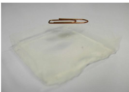
**Figure 6.10:** Aerogel material of low density with a paper clip on top. The top surface shows a dark grey spot caused by the impact of thousands of micron sized iron particles with a few  $\text{km s}^{-1}$ .
