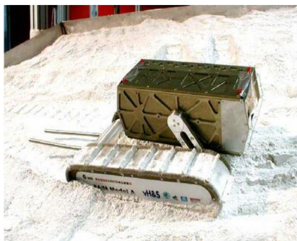
Figure: Nanokhod Microrover in dust analogue environment (Image courtesy by von Hoerner & Sulger GmbH)
