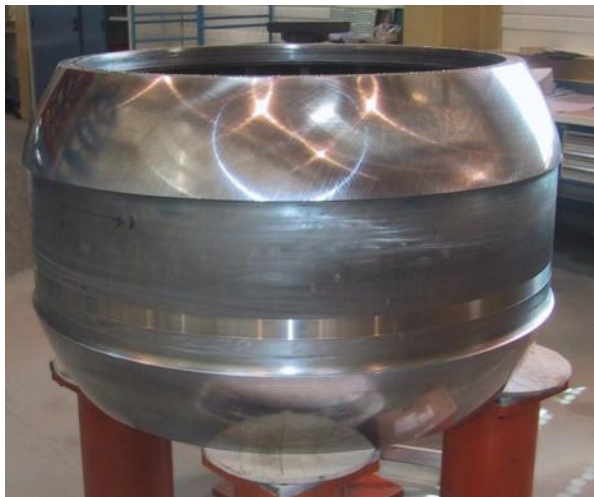
Fig. 14. The bearing sphere of the hydrostatic bearing.
