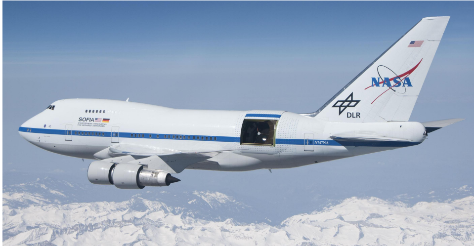
Fig. 1. SOFIA during a rare daytime test flight with the open cavity door in the aft fuselage. The telescope mirrors were protected with covers for these initial envelope expansion flights that were performed to proof the structural integrity of the fuselage after the extensive modifications.
