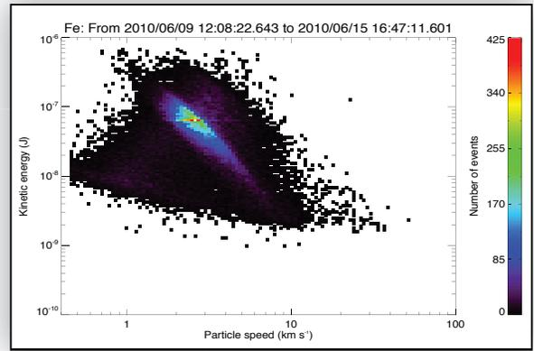
**Figure 32:** Velocity  $v$  and kinetic energy  $E_{\text{kin}}$  of accelerated iron micrograins to study impact effects at the dust accelerator.
