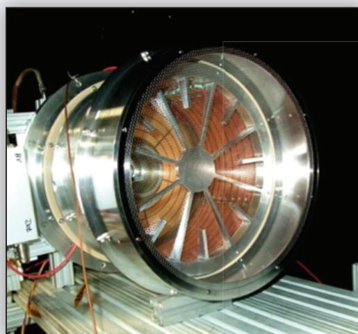
**Figure 24:** Laboratory model of the small dust telescope SUDA
