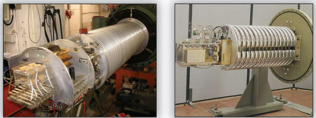
Figure 26: The Heidelberg 2 MV Van-de-Graaff accelerator (left) at the Max Planck Institute for Nuclear Physics, and the new 3.5 MV coaxial singletron accelerator (right) planned at the University of Stuttgart.
