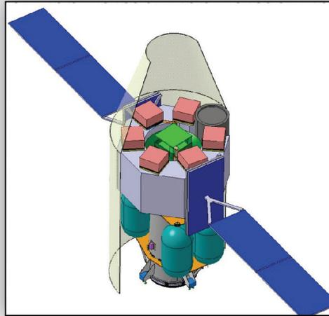
**Figure 37:** SARIM spacecraft in a VEGA payload fairing with extended solar sails (Astrium/EADS). Six Active Collectors (red cubes), one Dust Telescope (grey cylinder) and the collector sample stack (green) are mounted on the spacecraft body. The Sample Return Capsule encloses the collector samples in the centre (not shown).
