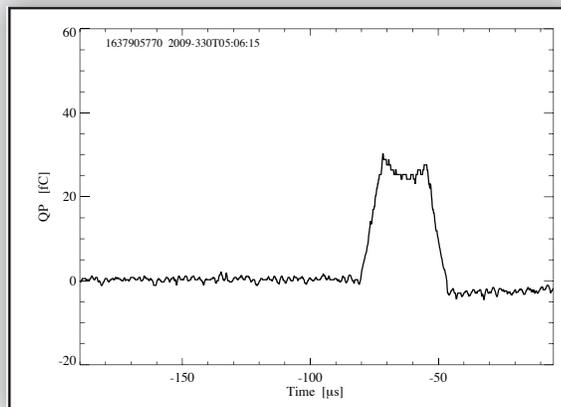
**Figure 15:** Induced charge signal of the CDA entrance grid channel (QP) due to a  $40 \mu\text{m}$  particle carrying an electric charge of 30 fC. The impact speed onto CDA was  $6 \text{ km s}^{-1}$  and this particle was detected in the Saturnian system in 2009. The impact occurred in the ring plane at a distance of 36 Saturn radii from Saturn.
