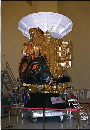
**Figure 12:** The Cassini-Huygens spacecraft in the clean room for Assembly Test and Launch Operations. The high gain antenna has a diameter of 4 m and the spacecraft has a wet (fuelled) mass of 5.6 tons. The CDA instrument with its white cover is mounted at the top left. Cassini was launched in October 1997 and reached Saturn in 2004 for orbit insertion. The end of the mission is planned for 2017.
