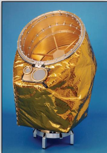
**Figure 13:** Flight unit of the Cosmic Dust Analyser for the Cassini mission. The instrument measures the speed, mass, electric charge and composition of individual sub-micron- and micron-sized dust impacts over a speed range of 1 to  $100 \text{ km s}^{-1}$ . The instrument has a mass of 17 kg and consumes 12 W.
