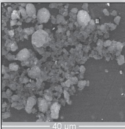
**Figure 31:** Electron microscope image of platinum-coated silica particles used at the dust accelerator.
