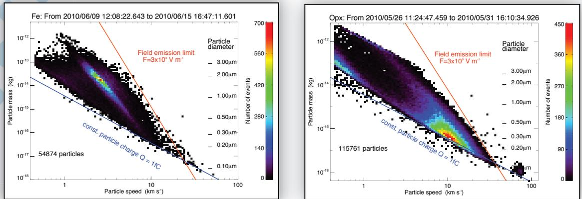
**Figure 30:** Velocity mass distribution for accelerated dust particles (left: iron, right: orthopyroxene). The blue line at the bottom determines the detection threshold of 0.1 fC and indicates particles with a constant charge. The upper red line represents a field emission limit of the grains of  $10^{10} \text{V m}^{-1}$  for grains with a constant field strength.
