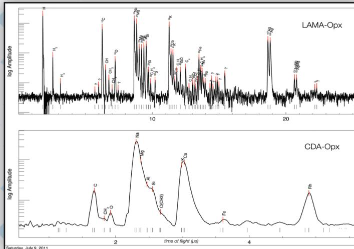
Figure 25: Comparison of the performance of the mass spectrometer CDA onboard Cassini (lower panel) and the new instrument LAMA (upper panel). The mass resolution of the new generation Dust Telescope is a factor of 10 higher.
