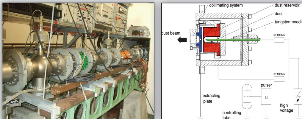
**Figure 29:** (left) Beam line of the dust accelerator with deflection electrode and electronics of the PSU. (right) Schematics of the dust source DS2001. A cavity is filled with submicron-sized grains and a pulsed high voltage of 20 kV between the reservoir and a needle lifts individual particles which leave the source through a central hole. This type of dust source is optimised for dust particles with low surface potentials, such as polypyrrole-coated silicates.
