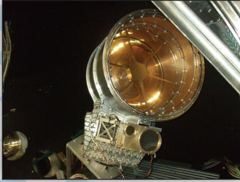
**Figure 28:** The Flight Spare Unit of the Cosmic Dust Analyser in the thermal vacuum chamber for dust accelerator tests at the Heidelberg accelerator facility.
