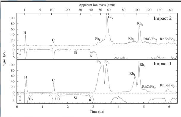
**Figure 16:** CDA Chemical Analyser time of flight mass spectra of two interplanetary dust particles. For clarity the spectra are shown inverted and magnified. The magnified view of the Impact 1 spectrum is magnified by a factor of 9, that of Impact 2 by a factor of 4.5. Carbon and Hydrogen are common contaminants of the Rhodium impact target but may also occur in the interplanetary dust particles
