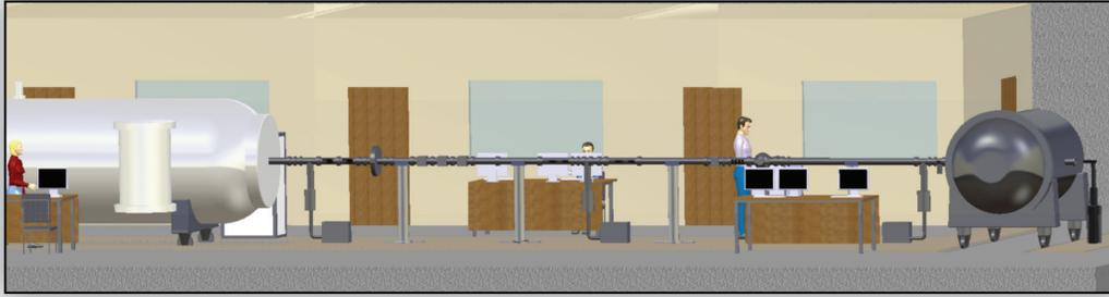
Figure 27: Concept of the new 3.5 MV Cockroft-Wolton Dust Accelerator providing micron and submicron dust grains with speeds between 1 and 100 kms<sup>-1</sup>.
