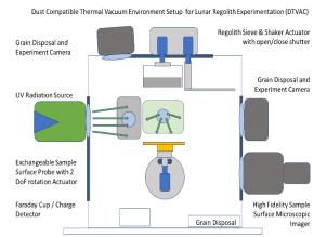
This thesis focuses on designing a test bench that simulates the lunar surface environment within a Thermal Vacuum (TVAC) chamber, based on an existing low-fidelity test bench. The design involves selecting test instruments such as a Camera/Microscope, lighting elements, and sensors. The test bench must comply with the NASA-STD-1008 standard.
